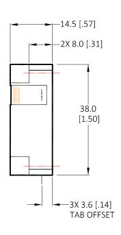
Body Housing: Steel, Nickel plated Tab Lead: Be-Cu, Silver plated
