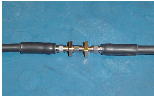
Figure 5: Maury 8021C21 and 8021A2 connected for “transmission” portion of calibration sequence.
